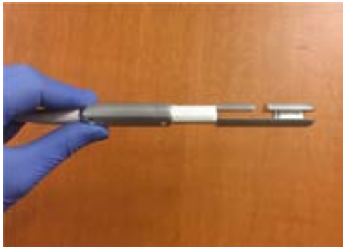
FIG. 5 Ann Arbor, USA, dynamometer speculum. Note that the bills of the speculum are covered by a condom when in use (reproduced with permission from J.A. Ashton-Miller, R. Zielinski, J.O. DeLancey, J.M. Miller)
